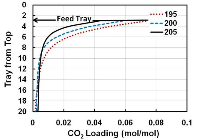
**Figure 4 Effect of Feed Temperature on CO<sub>2</sub> Loading Profile**
