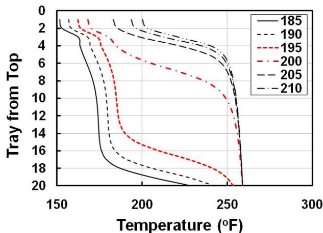
Figure 1 Effect of Feed Temperature on Regenerator Temperature Profile
