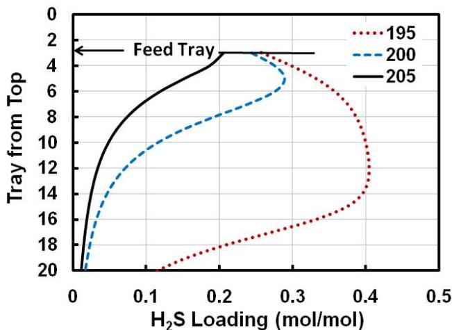
**Figure 3 Effect of Feed Temperature on H<sub>2</sub>S Loading Profile**
