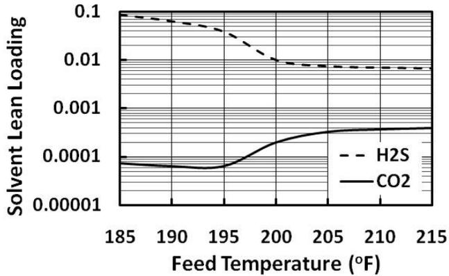
**Figure 2 Effect of Feed Temperature on Solvent Lean Loadings**
