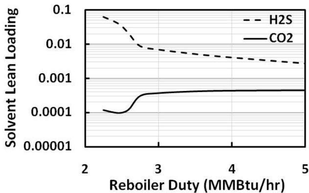
**Figure 2 Effect of Reboiler Duty on Solvent Lean Loadings**
