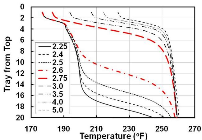
Figure 1 Effect of Reboiler Duty on Regenerator Temperature Profile
