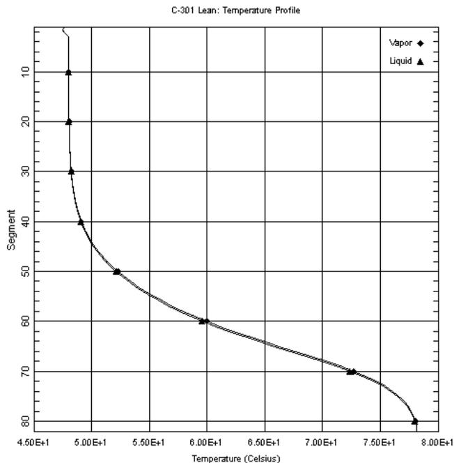
Figure 3 “C-301 Lean” Temperature Profile with Semi-lean at 78.0°C
