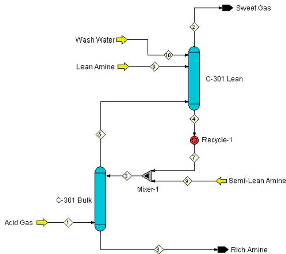
Figure 1 Two-Stage Absorber for CO<sub>2</sub> Removal in an Ammonia Syngas Plant
