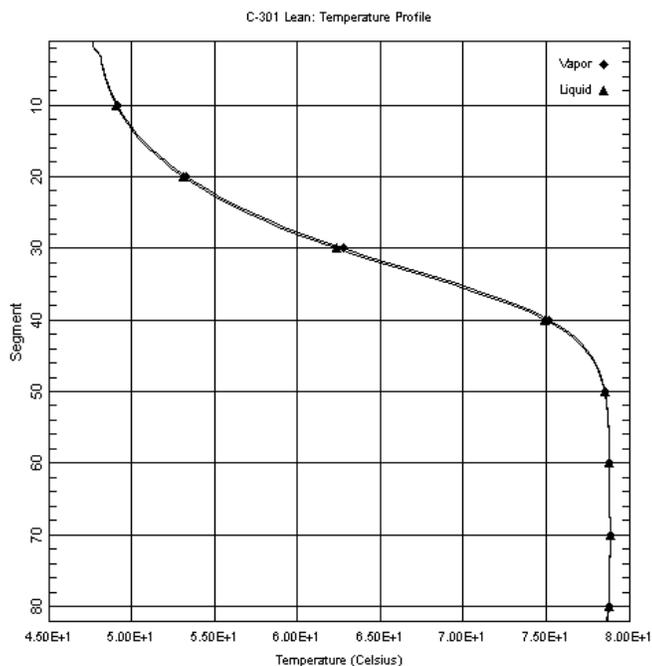
Figure 4 “C-301 Lean” Temperature Profile with Semi-lean at 78.25°C
