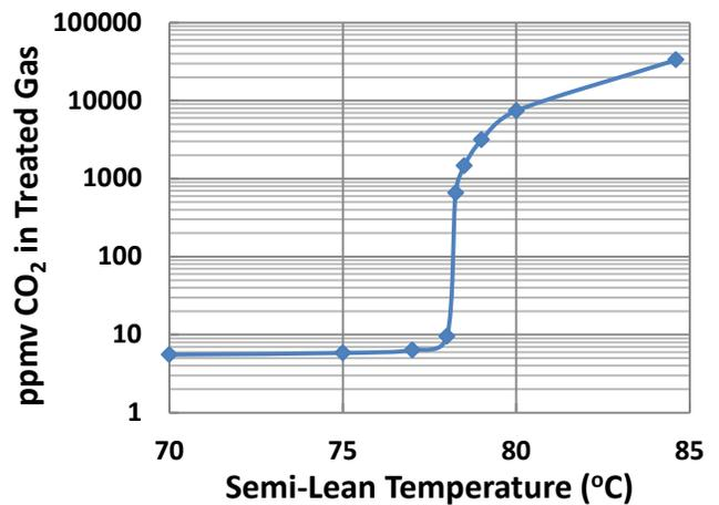
Figure 2 Effect of Semi-lean Temperature on Performance of 2-Stage Absorber
