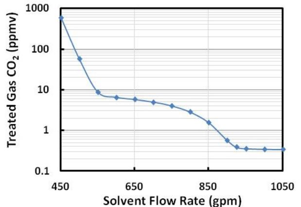
Figure 5 Performance of a Trayed LNG Absorber with 0.015 Lean Loading
