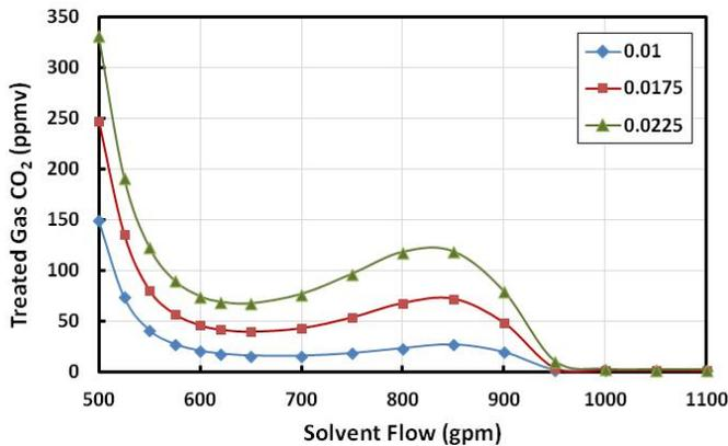
Figure 1 How Absorber Performance Depends on Amine Rate at Various Lean Loads
