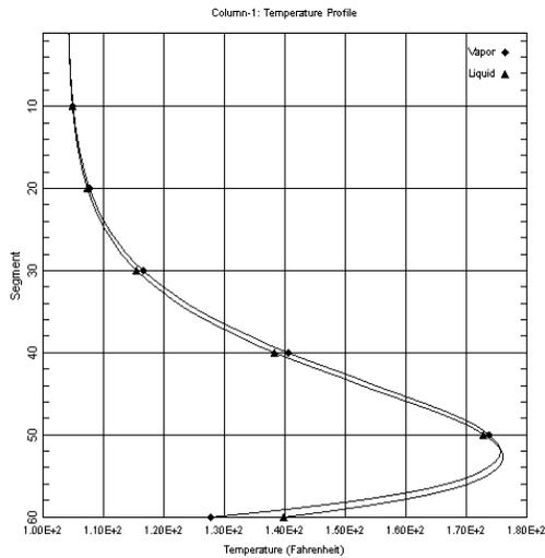
Figure 4 Temperature Profile at 1,000 USgpm
