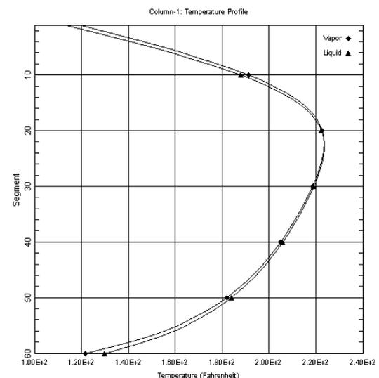
Figure 3 Temperature Profile at 800 USgpm
