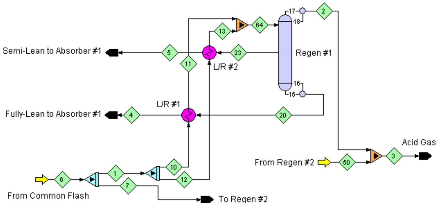
Figure 1 A Single Regenerator in a Parallel Train Split-Flow Amine System
