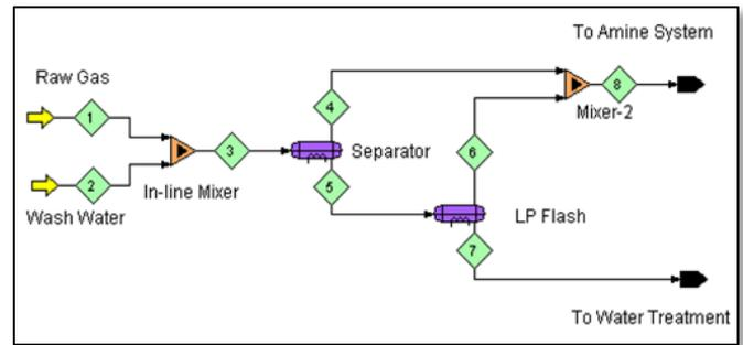
**Figure 3 Water Wash Scheme for MeOH Removal**
