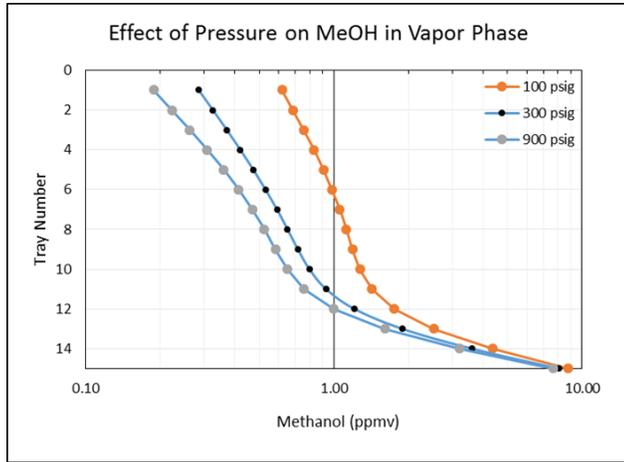
**Figure 1 MeOH Removal vs. Absorber Pressure**
