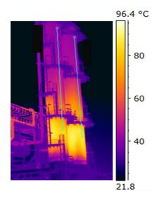
The bulge temperature was still warm (80–85°C) but the peak was in the bottom part of the towers where they are stainless steel clad so there are no corrosion concerns. Incidentally, the measured and simulated CO<sub>2</sub> levels in the treated gas were 2 ppmv and 1 ppmv, respectively.
