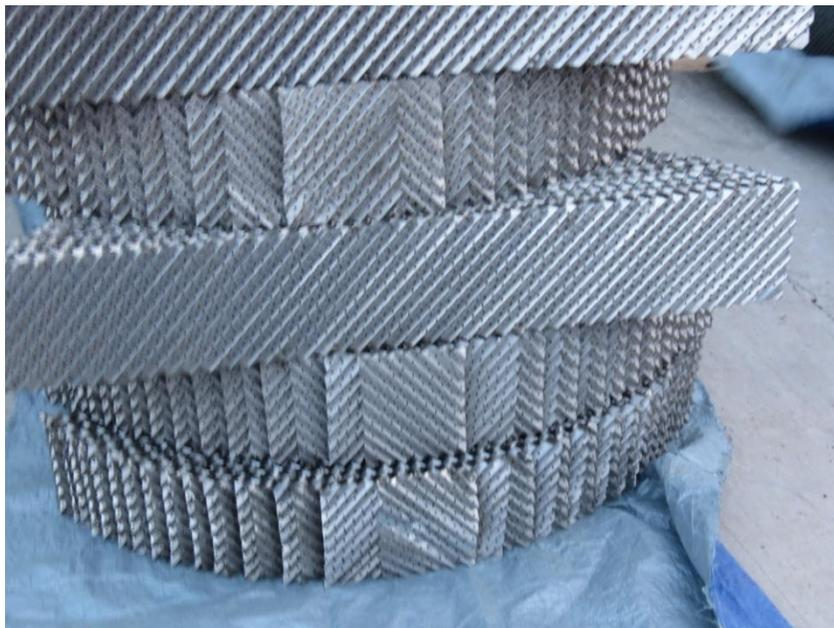
**Figure 1** Structured Packing Bricks Used in Revamp
