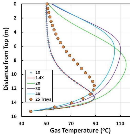
**Figure 3 Absorber Temperature Profiles for Various Packing Sizes and for Trays**
