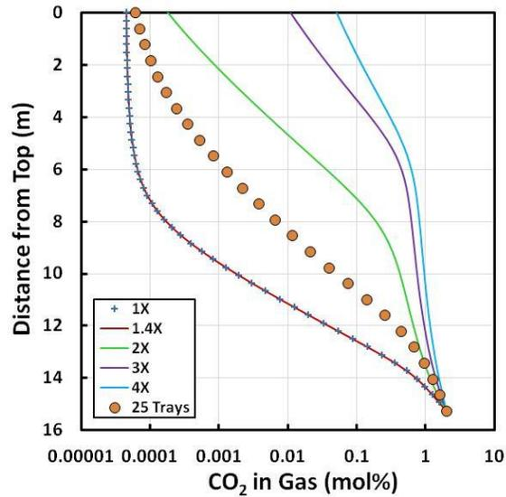
**Figure 2 Absorber CO<sub>2</sub> Profiles in the Gas for Various Packing Sizes and for Trays**
