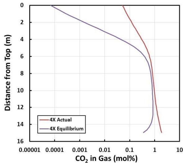
**Figure 5** Actual and Equilibrium CO<sub>2</sub> Concentrations in the Gas at Various Positions in the Absorber. Packing is FLEXIPAC® 4X.
