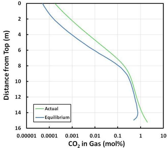
**Figure 4** Actual and Equilibrium CO<sub>2</sub> Concentrations in the Gas at Various Positions in the Absorber. Packing is FLEXIPAC® 2X.
